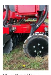
2 Rows of Serrated Discs on Rubber Torsion Bars
