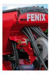
1,000 L Hopper with Accord Metering Unit and Electric Metering
