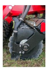
Hardened Seed Tube with Weaving Rubber Exhaust Boot
