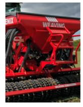
Folded rear loading step with a security hand-rail & LED road lights
